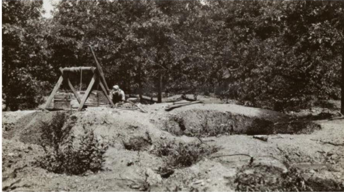
B. Miner using windlass to hoist ore from shaft; abandoned shaft and waste piles nearby
