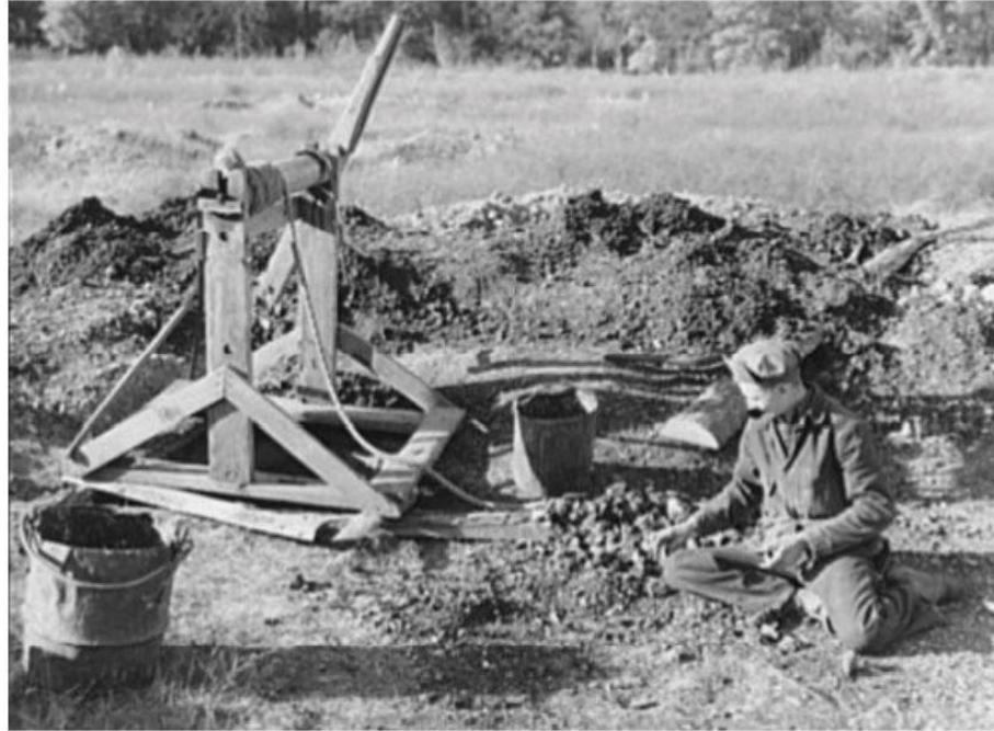
B. Miner sorting and cleaning barite ore next to shaft and windlass
